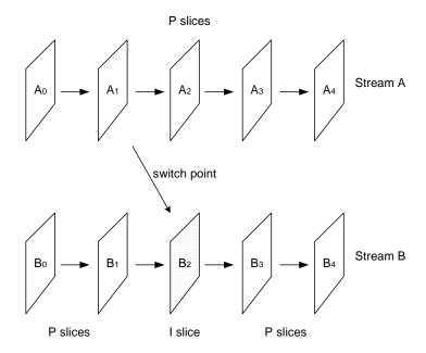
Figure 2-1 Switching streams using I-slices
