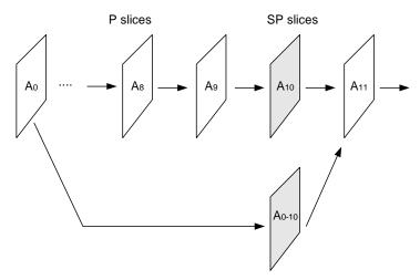
Figure 2-8 Fast-forward using SP-slices
