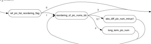
If ref\_pic\_list\_reordering\_flag is 1, the reordering process is repeatedly carried out until reordering\_of\_pic\_nums\_idc is 3.
