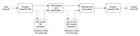
Figure 5-1 Transform, quantization, rescale and inverse transform flow diagram
