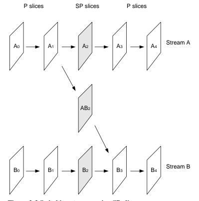
Figure 2-2 Switching streams using SP-slices
